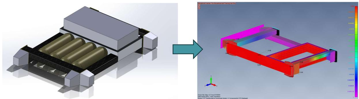
One of the coursework designs I have modelled was to create a FCEV composite chassis and have it simulated in Siemens Femap. Performing both front and side impact where made to test not only the durability of the design but also the effectiveness of the added attenuators.
