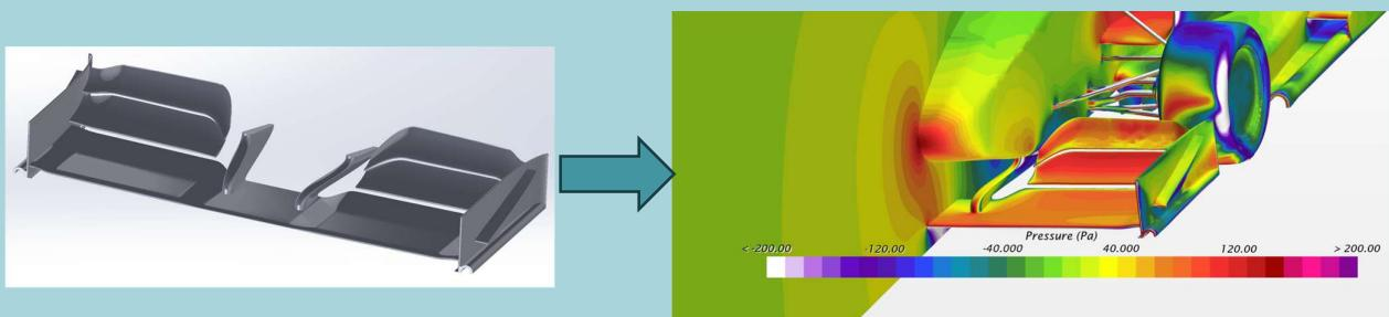
This Front wing update was added to simulate the effect of the flow with the mounts and simplify the overall assembly with the new design target to maintain aero balance. This simplification was also, as a result of the 1.4 iteration which shows a loss in performance with curved cascade flaps.
