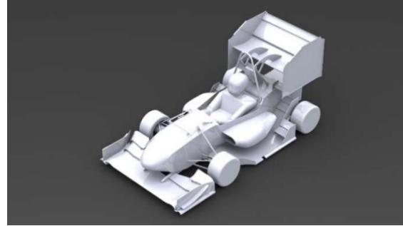
As coordinator for the design phase of the 2024 Aero subsection, this design was focused on implementing simplistic manufacturable venturi with existing wing elements. Utilizing as much of the existing elements from previous years culminating in an all-new aero package.
