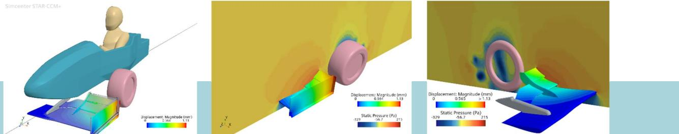
This Dissertation involved taking the established design for the Oxford Brookes Racing 2025 Front wing and validating it in a fluid-structure interaction simulation, which simulates the Stress analysis and Fluid Flow simultaneously to provide instant feedback and the change of the front wing while illustrating the impact on the aerodynamics.
