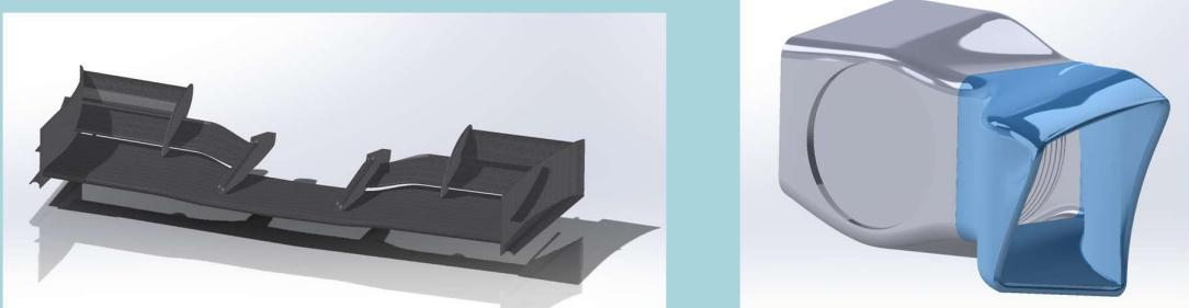
First is the front wing planned for this years package with an enlarged endplate design iteration to reduce disruptive flow to devices behind. Second is the front air-cooled ducting inlet for the unsprung motors, aimed at directing more flow from the angled front wing to the heatsink inside the cover.
