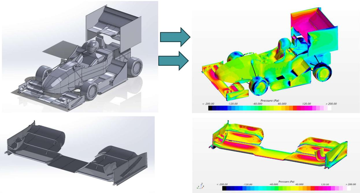
The Design team which I coordinated was set up to develop a design to remove the previous sidepod design and incorporate the same radiators into the side wing venturi. Along with the new side wing design another one of the responsibilities was to design and validate a new front wing.
