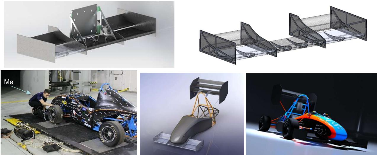
As Aerodynamics Department leader for 2020 and 2021 year cars an Aero package was developed employing new manufacturing techniques and automated validation for airfoil designs.
