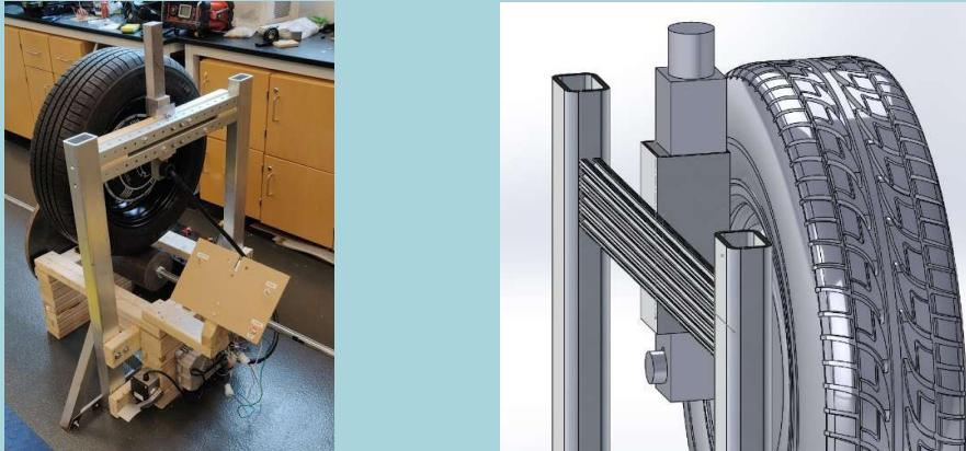
Above is the electric wheel testing platform design. A NSERC Research project to construct a platform for testing OEM in wheel electric motors performance parameters.
