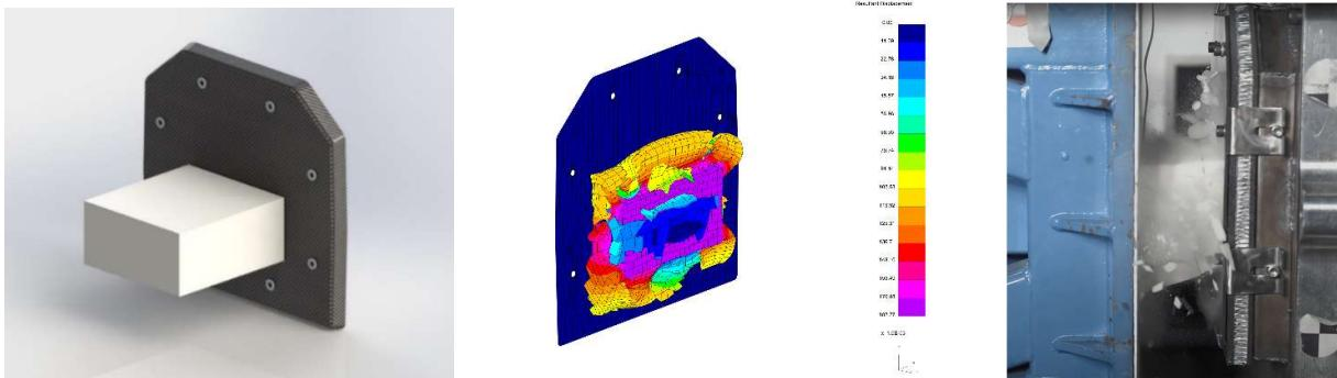
Involvement with Composites included the responsibility of implementing a composite anti-intrusion panel with testing done with Cranfield University Impact Centre.
